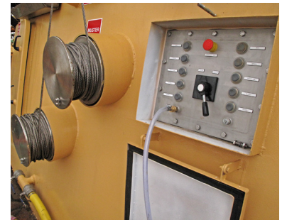
▲ The deck control box for the main winch and the two landing winch drums.
