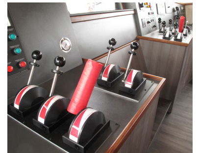
▲ The winch control levers are positioned each side of the central control position. The clutch levers for the safety drums keeping the block at the head of the derricks are padded.
