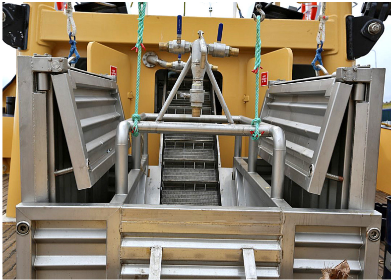
▲ The stainless steel bins on deck are opened out when fishing starts, with the codends emptied into them and the catch routed to the central conveyor. (Photo: Hanneke de Boer)
