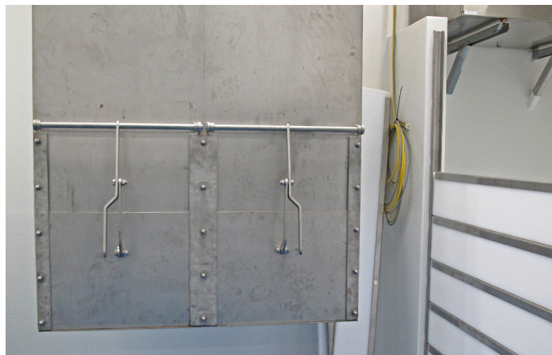
▲ Washed fish are routed via a chute to the two fish bins in the fishroom.
