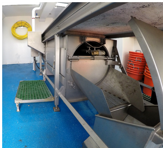
▲ The fish washer is built into the sorting conveyor under Georgina of Ladram's whaleback.
