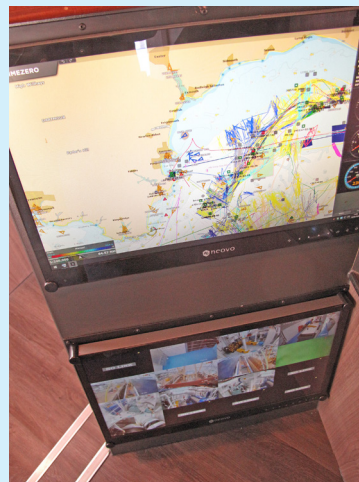
▲ The MaxSea TimeZero set and the CCTV monitor built into the control console.
